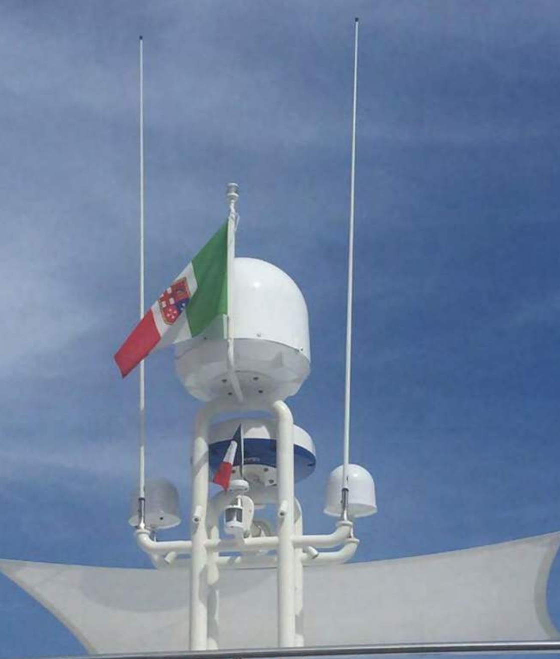
Glomex antennas - from left to right: 2.4m/8' High performing VHF antenna (model RA1225), weBBoat 4G Plus (the Dual Sim Coastal Internet antenna system), Rhea (47cm/18,5" DVB-S2 Satellite TV antenna), Altair (Full HD DVB-T2 TV antenna) and 2,4m/8' AM-FM radio antenna (model RA1288)
